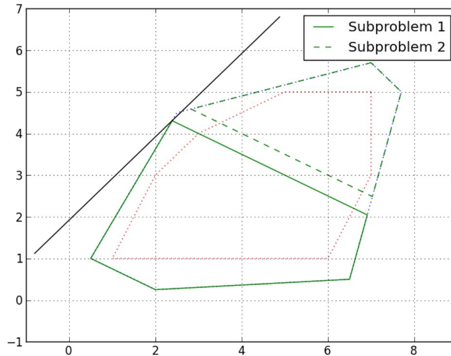
Figure 4: Branching on disjunction  $x + 2y \leq 11$  OR  $x + 2y \geq 12$
